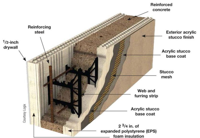
Figure 3 – Typical ICF Construction<sup>2</sup>
