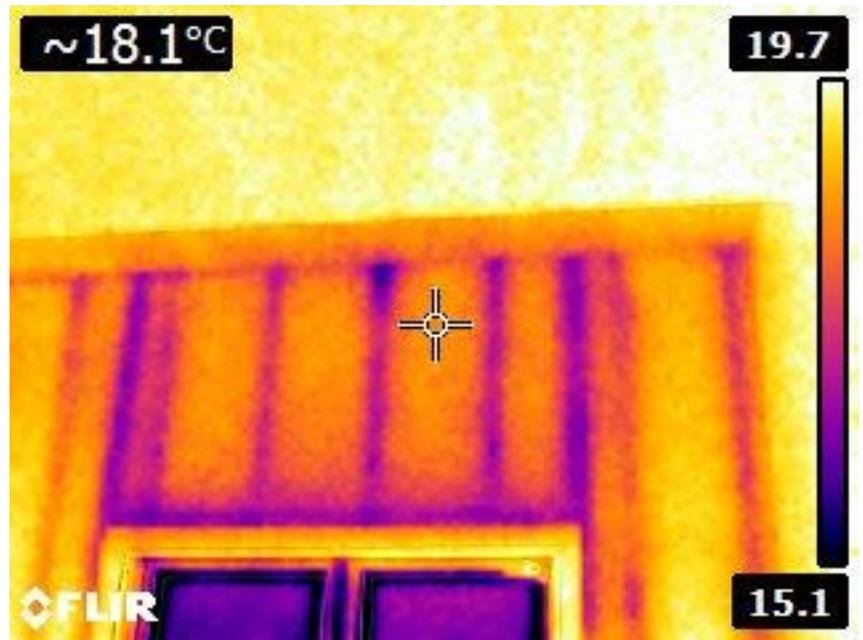
Figure 2 – Thermographic Image of a Steel Frame Construction
